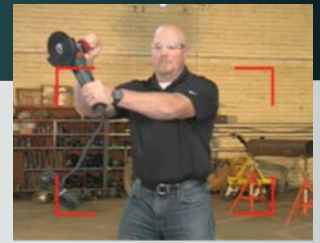
Personal Safety Cutting Zone: Keeping both hands on the grinder at all times
